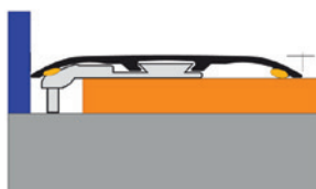
Fixation with adhesive + perimeter pin
