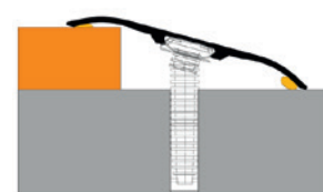
Fixation with adhesive + screw anchor
